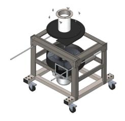
Before cleaning of the ventilator unscrew the winged screws and remove the upper flange from the ventilator.
