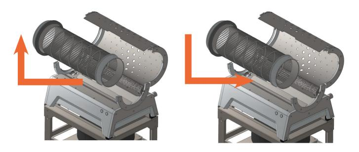
4. Close the upper frame of the device and secure the locks in the correct position
