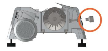
Before cleaning of the knife unscrew the knob so that the knife can be tilted.
